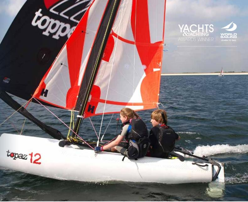
Safety features include a fully sealed mast and masthead float to ensure that should the 12 be capsized it will float on its side rather than inverting. Righting lines and weight placed aft on the hull means righting the boat is effortless even for very lightweight crew.
