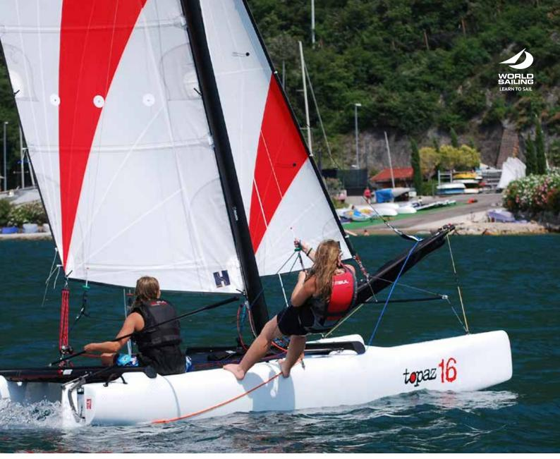
As with the 12 and 14, the skegs have been moved right under the mainsail where they act like centreboards that let the cat spin round so that the 16 tacks like a dinghy but won't fall over. The 16 is a sweet machine to drive with taut and responsive feedback proving that high performance rotomoulded cats have truly come of age.
